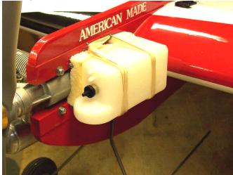
93. Plumb tank. Install propeller for your engine.
