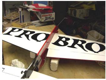
57. Aileron servo mounting (one method).
