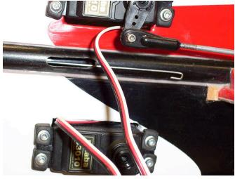
**52.** Tape wires with connectors staggered.
