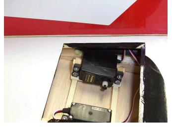
**79.** Attach throttle servo mount to the rails.
