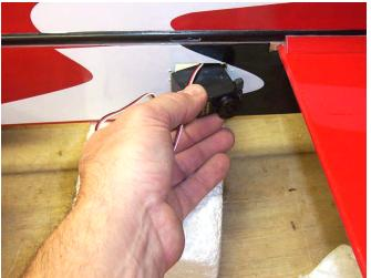
□ 43. Servo mounted with the pig tail out of the "goo trail".
