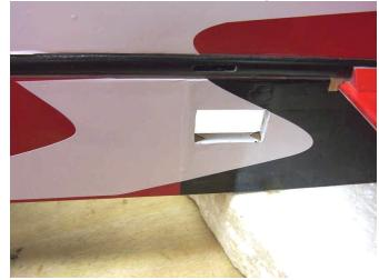
□ 42. Load the servo with the pig tail on the side of the servo.
