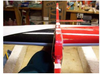
29. Use 30 minute epoxy with micro balloons. Make a nice thick paste. Drizzle the epoxy mixture in the joint.
