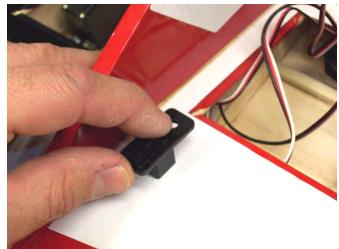
**70.** Cut the hole, pull the charge wire thru.
