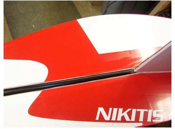
□ 31. Fill any gaps between the wing and fuse.
