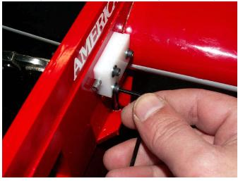
□ 39. Install wheels and collars. Flatten a spot on the axles and use locktite on collars.
