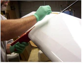
10. Put a little epoxy on the fuse. Apply from the wing saddle forward. We'll do the tube to fuse joint later.
