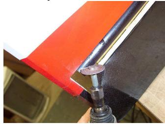
24. Cut the covering back a little and glue the first piece of tri stock to the stab on the mark 1/4" from the centerline.
