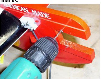
82. Drill the 2.5° Thrust Wedges (available at swanyshouse.com) for the motor bolt pattern.
