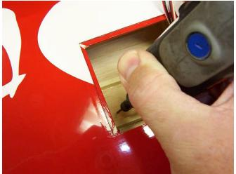
□ 60. Enlarge the hole just big enough to fit the servo output shaft.
