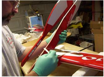
11. Line up the front of the fuse with the end of the motor mount.
