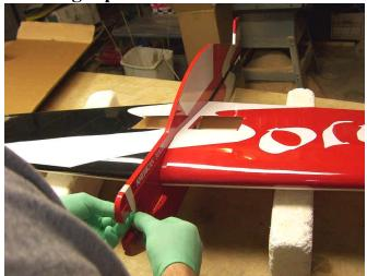
13. Slide in the landing gear mount before gluing the fuse on. Insert with tines pointing toward tail (not like the picture!).
