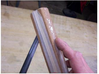
2. Glue the tube to the motor mount. Cut a little covering away so glue can bond to the wood.
