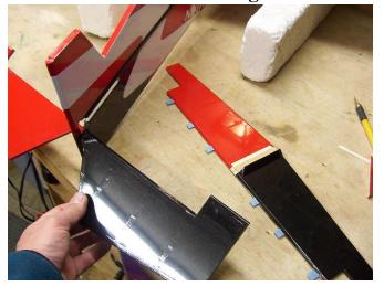
□ 26. Slide the hinges in before gluing. Then glue with some epoxy top and bottom.
