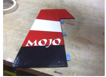
□ 34. Glue rudder hinges, check movement.
