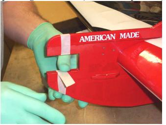
□ 14. Truing the Fuse. Tape the fuse to mount.
