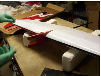
8. Open the holes in the landing gear mount with a soldering iron.
