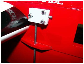
**38.** Tighten screws to hold gear firmly.
