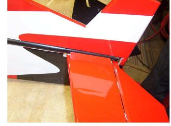
28. Make sure the horizontal stabilizer is level with the wing.
