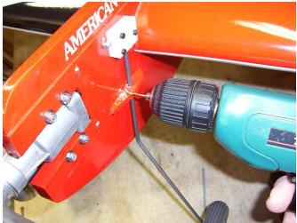
90. Insert some left over control rod into the holes.
