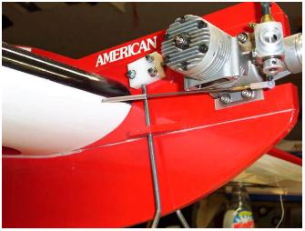
89. Fuel Tank Mounting (one method).Mark and drill 4 holes to attach the tank.
