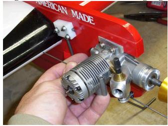
□ 87. Linkage to the servo. Easy connector shown.
