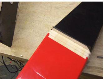
25. Hinge the stab to the elevator and slide in the elevator in the fuselage first.
