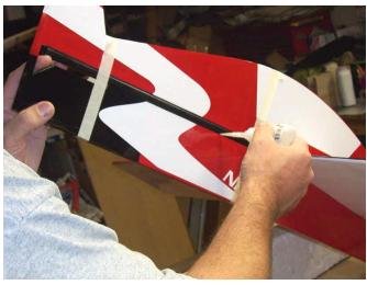
21. Mounting the Horizontal Stab. Mark the center of the stab.
